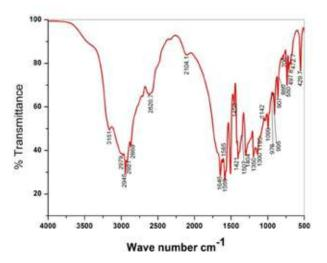
Fig. 3 FT-IR spectral band assignment of LLA single crystal
