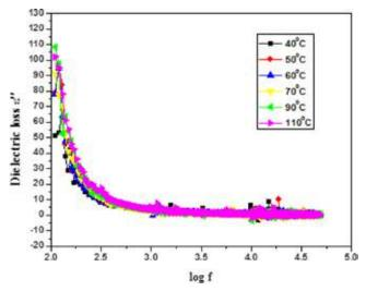
Fig. 7 Logarithmic relationship between dielectric loss and temperature
