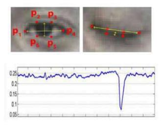
Figure 5. Automatic detection of landmarks p (i) for both open and closed eyes. Plotting the eye aspect ratio (EAR) from Eq. (1) over several frames of video
