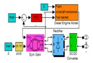
Fig. 8. MATLAB simulation design for DG modelling
