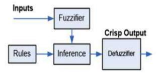
Fig. 13. A fuzzy logic system: (a) FLC's essential elements
