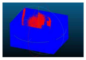
Fig 7. Point cloud after alignment of the scanned wall (RED) and the room (BLUE)
