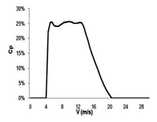
Fig. 4. Energy co-efficient versus varying wind speeds
