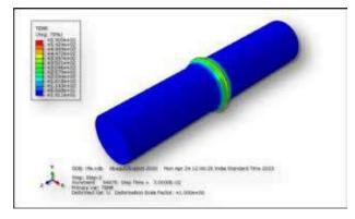
Fig. 2 Temperature simulated Model for the bars Experimentally recorded
