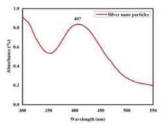
Fig. 1.UV-Vis spectrum of Silver nanoparticle
