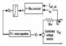
Fig. 11. Modelling & validation of supercapacitor SC: SC equivalent electrical circuit
