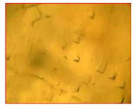
Fig. 12(a) Crystalline LLA surface etched for 5s as grown
