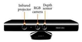
Fig 2. Xbox 360 Kinect Sensor[27]
