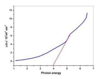
Fig. 5. Band gap diagram of LLA single crystal h against (αhv)2
