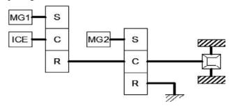
Fig.10 Mechanism of Hybrid Synergy Drive
