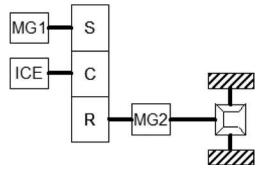
Fig.9 Mechanism of Hybrid Synergy Drive
