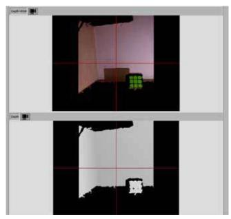
Fig 3. Output of RGB camera(top) and Depth Camera(below) of Kinect Sensor.
