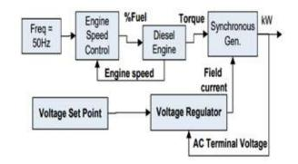
Fig. 7. Diagram of the DG model used for modelling
