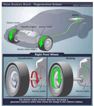
Fig.12 Regenerative braking system
