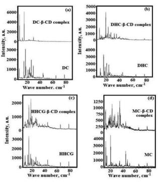
Fig. 3. Comparison on the X-ray diffraction pattern of free- and  $\beta$ -CD inclusion complex of (a) DC, (b) DHC, (c) HHCG, & (d) MC.
