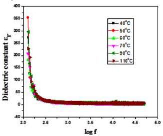
Fig. 6 Temperature dependence of the logarithm of the dielectric constant
