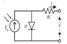
Fig. 2. Circuit model for a single-diode photovoltaic cell
