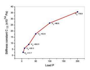
Fig. 11 Changes in the stiffness constant (C11) as a function of load P
