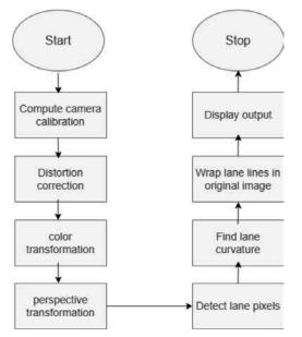
Fig. 1 Proposed architecture of LDS
