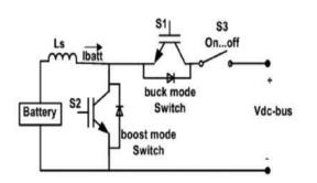
Figure 10. Battery storage system modelling and control: A diagram of the battery and the direct current (DC) bus control system
