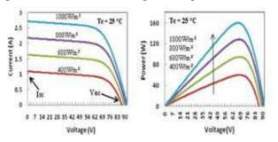
Fig. 3. Variable sun radiation and a cell the temp of 25 °C are aspects of the VI solar array model
