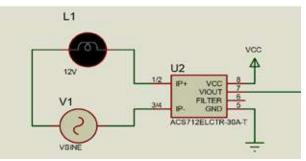
Fig. 4 Current Sensor Circuit
