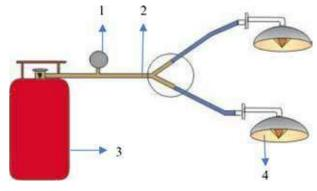
Fig. 3. Gas Brooder 1. Regulator, 2. Gas tube, 3. LPG Cylinder, 4. Gas Burner
