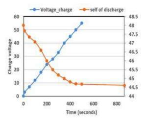
Fig. 12. Supercapacitor SC model creation and verification: it's charging as well as self-discharging performance
