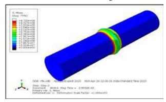
Fig. 3 Residual stress modal of Rotary Friction Welding of AA6061
