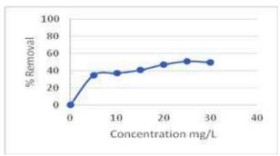
Fig. 2, Effect of initial solution concentrations (mg/lit)
