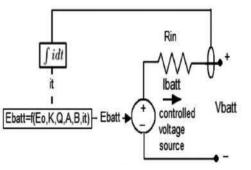
Fig. 9. An analogous lead acid battery electrical circuit is used for modelling and controlling battery storage systems
