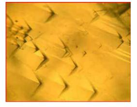
Fig. 12(b) Ten-second etching of an as-grown LLA crystal's surface
