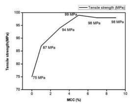
Fig.7. Tensile strength of the biocomposite film
