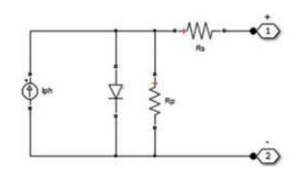
Fig. 2. Equivalent Circuit Model of PV Cell SHUNT ACTIVE POWER FILTER
