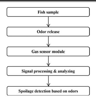
Fig. 1. Mechanism of developed EN system
