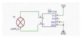
Fig. 3 Voltage Sensor Circuit Diagram
