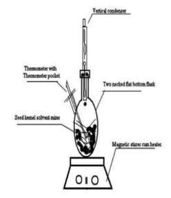
Fig 1: Experimental Set-Up for extraction of custard apple seeds
