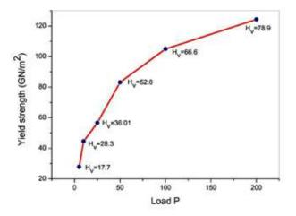
Fig. 10 Yield strength ( $\sigma$ y) vs load (P) as a function of time
