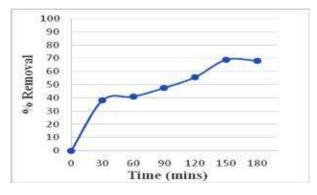
Fig. 3 Effect contact time on removal of Lead
