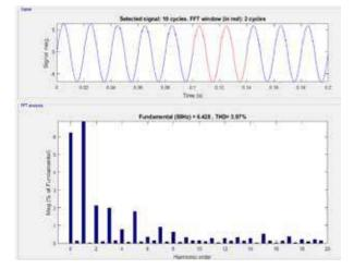
Fig. 5. Current with harmonics and THD with SAPF CONCLUSION
