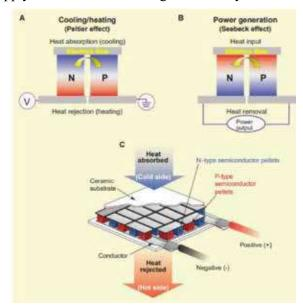
Fig 1. Working of Peltier plate
