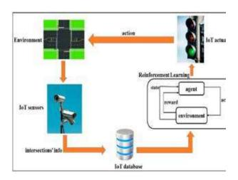
Fig. 2. IoT and ML approach for ATM
