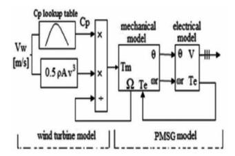
Fig. 5. Diagram of the WEG model's SimulinkSimPowSys simulation
