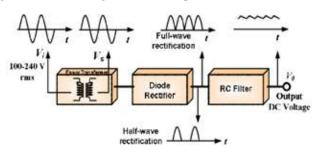
Fig. 5 DC Power Circuit Block Diagram
